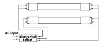
2) Connect two wires to branch circuit L and N according to the figure below.
