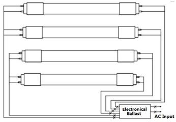
2) Connect two wires to branch circuit L and N according to the figure below.
