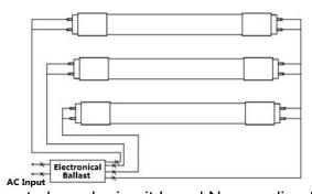
2) Connect two wires to branch circuit L and N according to the figure below.
