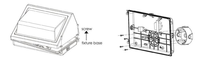
Method 2: Drill holes at the required three mounting points, mount the fixture by securing mounting screws (provided by others) through the drilled holes, and seal the screw heads with appropriate waterproofing material.
